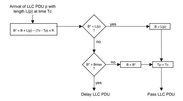
Figure 8.2: Conformance Definition Algorithm for BSSGP Flow Control
