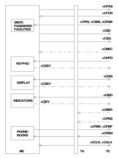
Figure 7: Mobile equipment control and status commands
